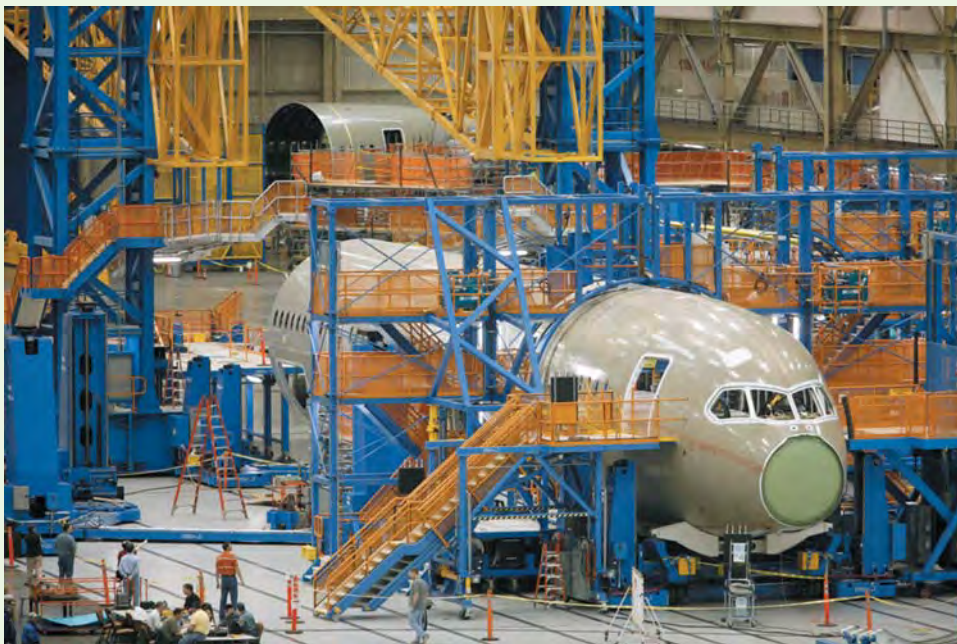
The first Boeing 787 Dreamliner takes shape in the final assembly plant in Everett, Washington. The new commercial airplane is assembled with major components produced worldwide.
